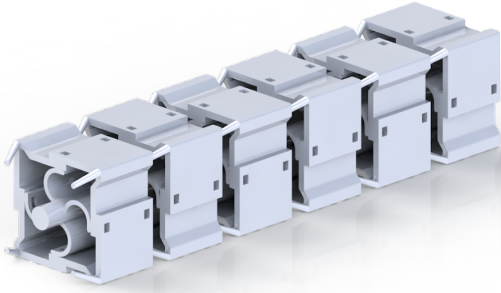
Fig. 5. CAD model of final body design with peg-socket linkages added between segments
